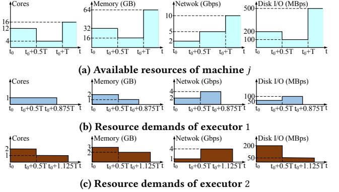
Figure 6: An illustration example of MinFrag . (a) The remaining resources of machine j until time t_0 + T , when a running executor will complete its execution. (b) The time-series resource usage of executor 1 which is expected to finish at time t_0 + 0.875T . (c) The time-series resource usage of executor 2 which is expected to finish at time t_0 + 1.125T . The capacities of machines are: 16 cores for CPU, 64 GB for memory, 10 Gbps for network, and 500MB/s for disk I/O.
